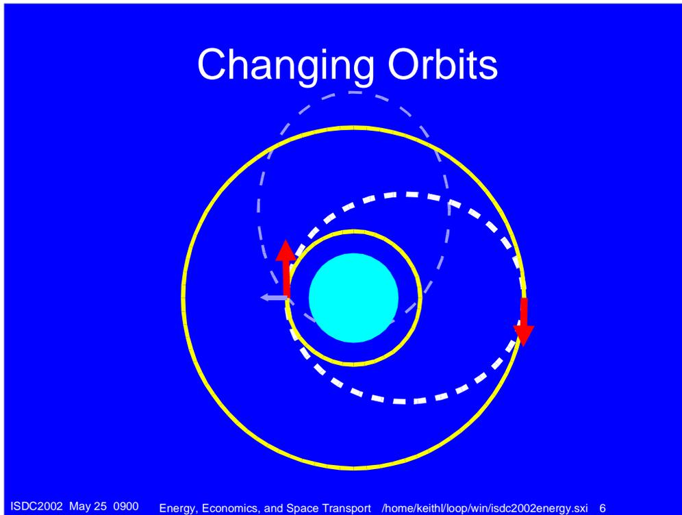
To get from anywhere to anywhere else involves changing orbits. To go from a low circular orbit to a high one involves two velocity changes, one HERE that puts you into an elliptical transfer orbit, and one OUT HERE that takes you out of the elliptical transfer orbit and injects you into a circular orbit.
